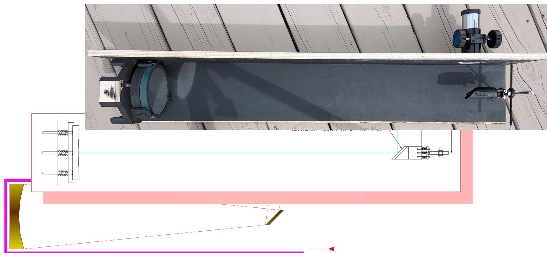
Concept, Plans and Construction of the Optical Part of the “First Light” Telescope
