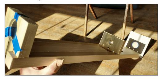
Above is a mockup of a solar projector I made from wood and some inexpensive lenses (less than \$10) from an online retailer called Surplus Shed. Here's the web address <a href="https://www.surplusshed.com/">https://www.surplusshed.com/</a>. The two lenses I used are on the site's front page. The bright round disc seen at the lower right is an image of the sun as seen through my window.
