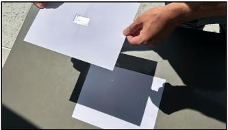
In this NASA image a pinhole through a bit of foil taped to a piece of cardboard, used as a sun shade, makes a tiny image of the Sun.
